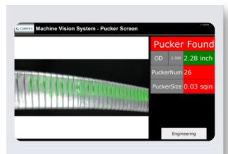
Puckering Detection System combines artificial intelligence and machine vision to detect armor deformation and puckering during cable manufacturing.
