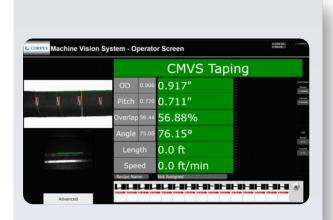
**Copper Taping Vision System** delivers high-speed, real-time inspection for coppertaped cable production.
